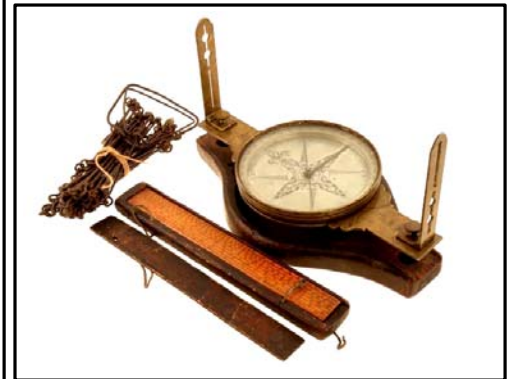
Early American survey tools consisted of a chain (20 links, that could be stretched to 66 feet), survey compass, slide rule, and rods (not pictured) (Courtesy American Philosophical Society) 3
